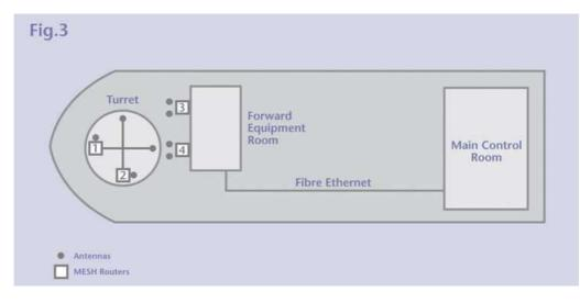
The connection to the Ethernet network is via 4 industrial switches running RSTP (Rapid Spanning Tree Protocol 802.11w) for providing redundancy in the Ethernet switches. It was decided to use standards based protocols rather than proprietary for the ease of integration and familiarisation with IT support personnel. If there is a failure in a switch it will find a new path to route the data in less than 2 seconds meaning little data is lost.
