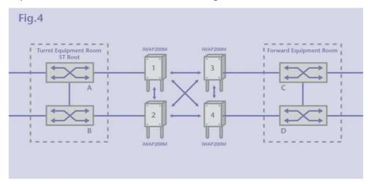
Choosing a MESH network architecture for this application also has another advantage in that it forms the basis of a backbone to allow other nodes to be connected around the vessel for other applications where an Ethernet device is to be connected, such as an IP camera for instance.
