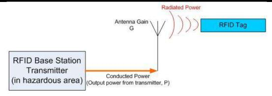
Actual radiated power = Conducted power in to the antenna, which is radiated in to free space
