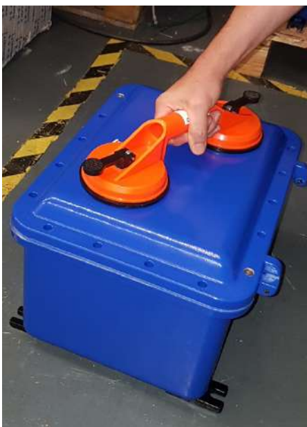
Figure 2: Opening iWAP107 Enclosure with Suction Lifter
