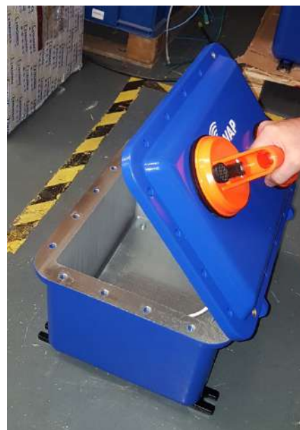
Figure 2: Opening iWAP107 Enclosure with Suction Lifter
