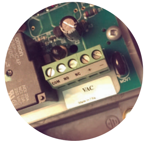
Figure R-7 DP-1C and DP-1D Terminal Block
