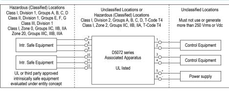
Associated Hazardous Area/ D5072 must Apparatus Hazardous Locations Terminals be Parameters **Device Parameters** Uo / Voc = 7.2 V ≤ Ui / Vmax Ch1 7-8-9 lo / lsc = 16 mA li/ Imax ≤ Ch2 10-11-12 Po / Po = 27 mW ≤ Pi / Pi
