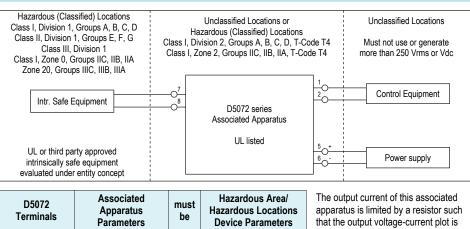
Uo / Voc = 7.2 V ≤ Ui / Vmax Ch1 7-8 lo / lsc = 23 mA li/ Imax ≤ Po / Po = 40 mW ≤ Pi / Pi
