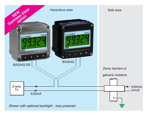
The BA324G loop powered 4/20mA indicator is an intrinsically safe field mounting instrument with a large 5 digit display housed in a robust IP66 GRP or stainless steel enclosure.
