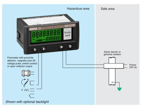
**The BA337E** is a third generation intrinsically safe rate totaliser that has similar functions as the BA338E, but is housed in a smaller 96 x 48mm DIN enclosure. The totaliser is easy to use and can be configured on-site to operate with flowmeters having a magnetic pick-off, switch contact, proximity detector, open collector or a voltage pulse output. A slide-in scale card simplifies identification and international intrinsic safety certification permits worldwide installation.
