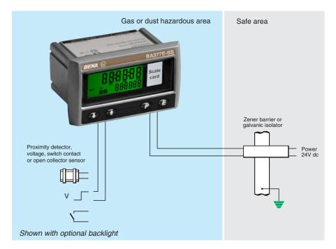
The BA377E-SS is an intrinsically safe instrument with one input housed in a rugged stainless steel enclosure that may be configured as a Timer or as a Clock. The intrinsic safety certification and the rugged enclosure allow the BA377E-SS to be safely installed in an Ex e, Ex p or Ex t panel enclosure without invalidating the panel enclosure's certification.
