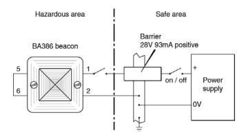
Fig 4 Using a single channel barrier.
