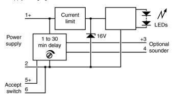
Fig 1 Simplified block diagram
