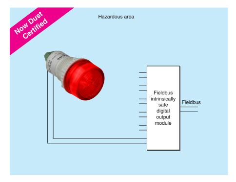
BA390S low current panel lamps provide reliable, cost effective visual status indication in all gas and dust hazardous areas. Each BA390S lamp produces a uniform output with just a few milliamps of input current and has a typical life greater than ten years.
