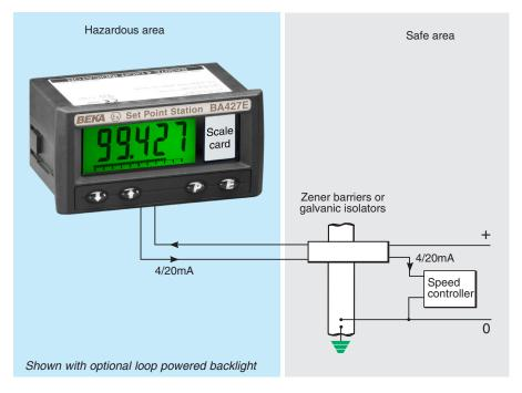
The BA427E is an intrinsically safe panel mounting set point station that enables the current flowing in a 4/20mA loop to be manually adjusted via the front panel push buttons from within the hazardous area. It is a second generation instrument that is mechanically and electrically compatible with the earlier BA405C, but has more display digits plus additional functions.
