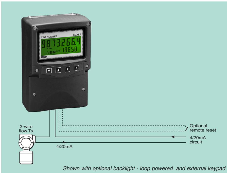
The BA554E loop powered 4/20mA rate totaliser is a third generation, general purpose, field mounting instrument that is electrically and mechanically compatible with the earlier BA554D, but it has a larger display, extended operating temperature and additional features such as a lineariser and bi-directional flow capabilities. Like its predecessor the BA554E is housed in a robust IP66 GRP enclosure with a separate terminal compartment
