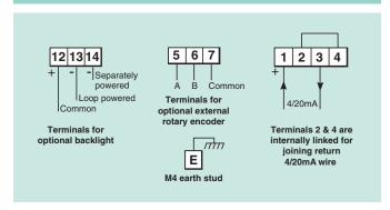
External encoder BA490 panel mounting rotary quadrature
