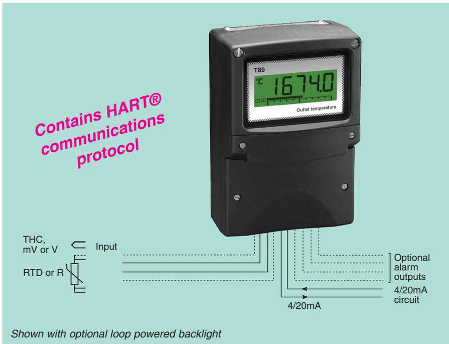
The new **BA674D** is a second generation, loop powered indicating temperature transmitter which replaces the BA574C. It provides an accurate local digital temperature display, plus a 4/20mA output, which may be scaled to represent any temperature range. Incorporating new facilities such as HART® digital communication and a robust GRP enclosure with a separate terminal compartment, the BA674D remains electrically compatible with the earlier model.
