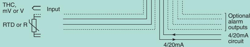
The new **BA678C** is a second generation panel mounting, loop powered indicating temperature transmitter which replaces the BA578C. It provides an accurate local digital temperature display, plus a 4/20mA output, which may be scaled to represent any temperature range. Although incorporating new facilities such as HART® digital communication, diagnostics and a robust enclosure with a IP66 front panel, the BA678C remains electrically compatible with the earlier model.
