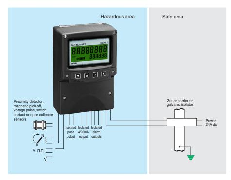
**The BA314E** is a third generation intrinsically safe field mounting tachometer housed in a robust IP66 GRP enclosure. The BA314E supersedes the BA364D. The tachometer is easy to use and can be configured on-site to operate with a magnetic pick-off, switch contact, proximity detector, open collector or a voltage pulse sensor. International intrinsic safety certification permits worldwide installation.
