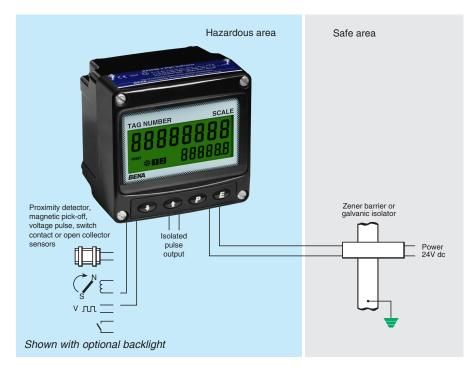
The BA314G is a third generation intrinsically safe field mounting tachometer housed in a compact IP66 GRP enclosure. The tachometer is easy to use and can be configured on-site to operate with a magnetic pick-off, switch contact, proximity detector or open collector sensor. International intrinsic safety certification permits worldwide installation.
