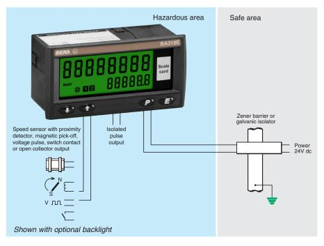
The BA318E is a third generation intrinsically safe tachometer that is compatible with the earlier BA368C, but has a much larger display and an isolated synchronous pulse output. The tachometer is easy to use and can be configured on-site to operate with a magnetic pick-off, switch contact, proximity detector, open collector or a voltage pulse sensor. A slide-in scale card simplifies identification and international intrinsic safety certification permits worldwide installation.
