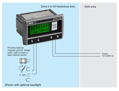
**The BA367NE** has a rugged stainless steel enclosure with Ex nA and Ex tc certification allowing it to be safely installed in an Ex n or Ex tc panel enclosure located in Zones 2 and 22, without the need for Zener barriers or galvanic isolators. The counter is easy to use and can be configured on-site to operate with a wide variety of sensors. A slide-in scale card simplifies identification.
