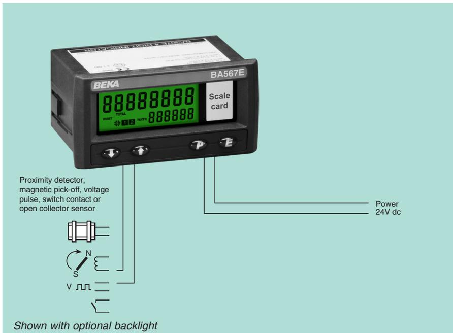
The **BA567E** is a general purpose counter with one input housed in a 96 x 48mm DIN enclosure. The counter is easy to use and can be configured on-site to operate with a magnetic pick-off, switch contact, proximity detector, open collector or a voltage pulse sensor. A slide-in scale card shows the units of measurement.
