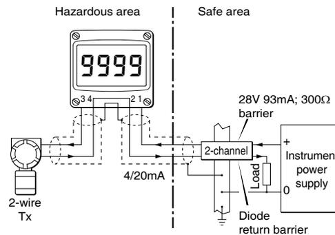
Fig 3 Typical measurement loop
