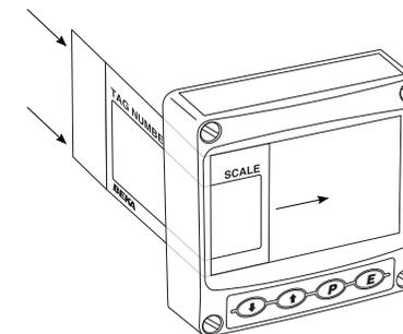
Fig 4 Inserting scale card into the instrument assembly.
